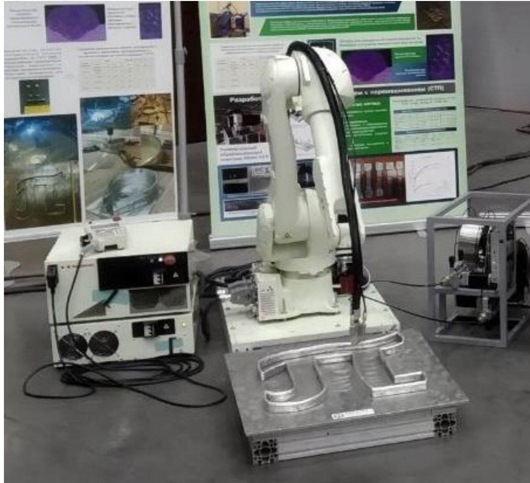
Double wire feeding system for welding, deposition and additive manufacturing
